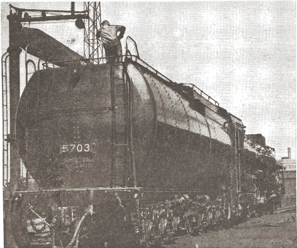
POWER for the International Limited , Montreal-Chicago pool train, is Hudson Type. These K-5-as, built in the Montreal Shops in 1930, are distinguished by smoke deflectors. Here the 5703 draws up for a long drink of water
