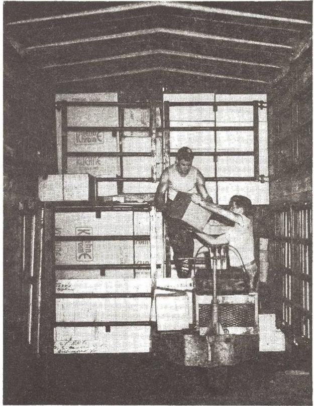
STEEL GRADES located at six foot intervals form bulkheads in new PRR boxcar protecting LCL shipments from damage
